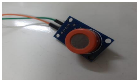
Fig -12: Gas Sensor
