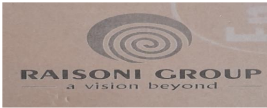
Fig-3[4]: LASER Engraving on cardboard
