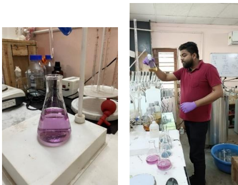
Fig. 4 The MICP treatment procedure is used to prepare and test UCS and STS samples.
