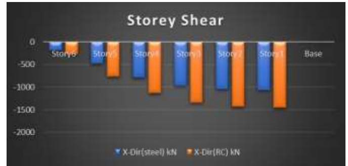
Chart -5: Storey Shear of both building in X- direction in response spectrum analysis.
