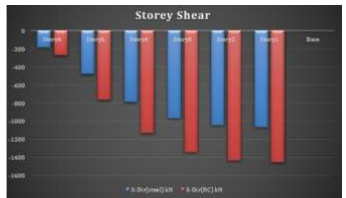
Chart -6: Storey Shear of both building in Y- direction in response spectrum analysis.
