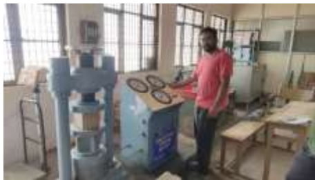
Fig.11 Compression test on concrete blocks
