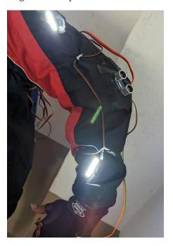
An innovative addition to the suit's architecture is the ultrasonic sensor embedded within the elbow region. This sensor employs high-frequency sound waves to detect obstacles and potential hazards in real-time. By constantly monitoring the immediate surroundings, the suit's user is alerted to any impending collisions or obstructions, mitigating risks and enhancing overall safety during operation.
