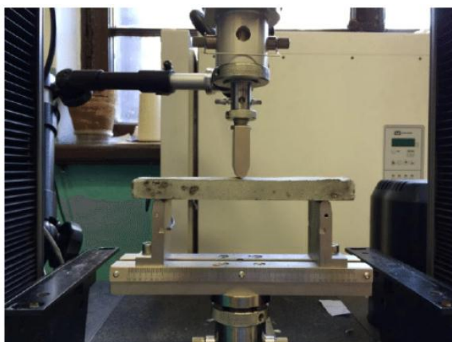
Fig. 5 Three-point bending test of concrete
