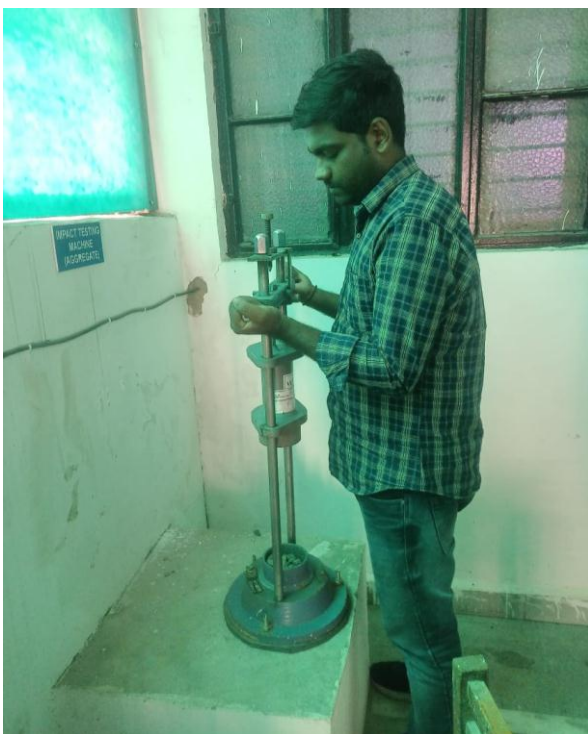
Fig. 1 Impact Test on the Coarse aggregates
