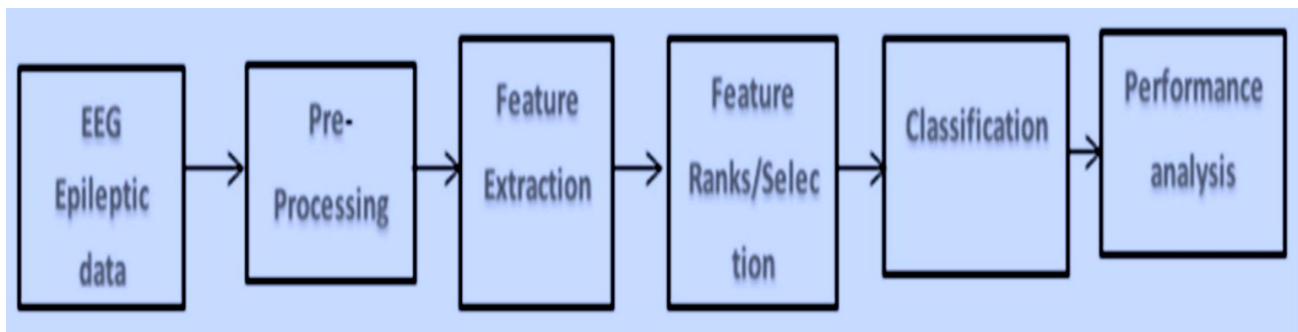
Fig. 3: Block diagram of an epileptic seizure detection system
