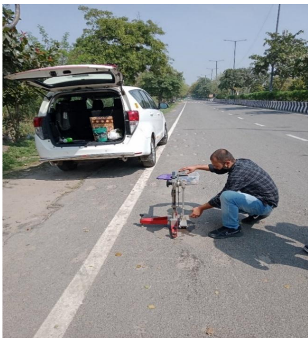
Fig -2: Data collection using British Pendulum Tester
