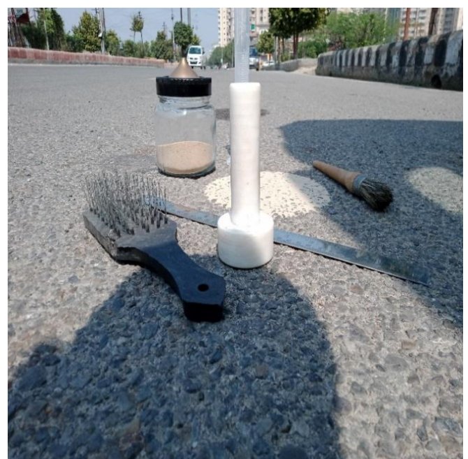
Fig -4: Sand Patch Test
