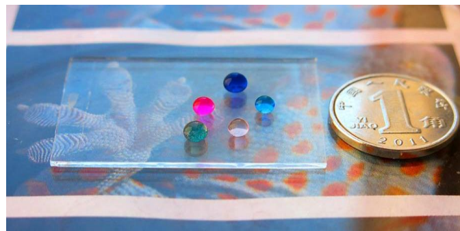
Fig -3.10: Optical photograph of spherical water drops on T-3 superhydrophobic coating [23].
