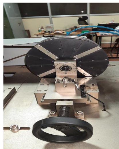
Fig -5: Side view of air foil bearing thrust rig
